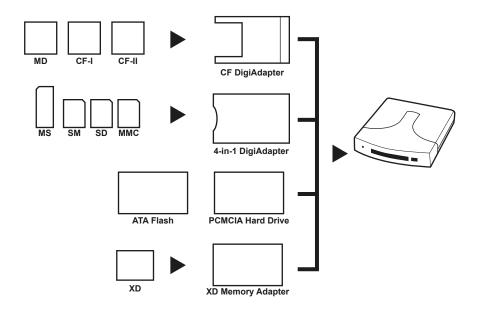
Note: The Pocket UDD ii is not compatible with Wireless Broadband card, Panasonic P2 card, SRAM card and Linear Memory card.
